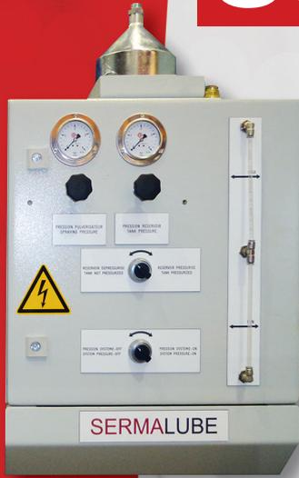
The micro-lubrication system **SERMALUBE®** has been designed and developed by **SERMAS®** for optimum lubrication for high-speed cutting applications (sheet, plate, ingot, billets) and surfacing aluminum plates.
